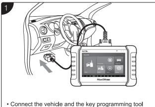
Connect the vehicle and the key programming to with the supplied main cable.
