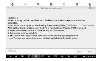
Figure 7-5 Sample Calibration of the Angle Sensor Screen 1
