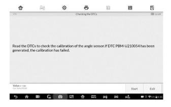
Figure 7-8 Sample Calibration of the Angle Sensor Screen 4
